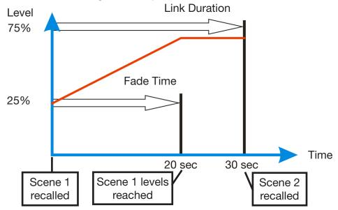
In this example, the levels start at 50%, and Scene 1 sets the levels to 75%. Fade Time is 20 seconds and Link Duration is 30 seconds.
