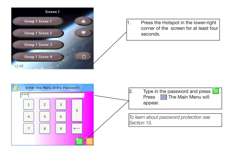
When you have entered a valid password, features protected by the password can be used until the password expires. The password expires if you return to a Screen, and do not return to the Configuration menus within 20 seconds. After this time, if you want to access the Configuration menus you must enter the password again. This ensures that TouchPanel's Configuration menus are protected automatically from accidental or unauthorized access.
