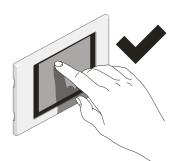
TouchPanel uses a touch-sensitive screen designed for use with your fingertip or a stylus. To select an item on the screen, press once on the item, using gentle pressure.
