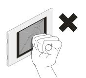
TouchPanel is designed to withstand mild impacts, but it may be damaged if struck too hard. You need only press the screen gently to select an item. As a simple rule, if the picture becomes distorted when you press the screen, then you are pressing it too hard.
