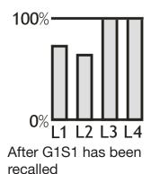
Next, when Group 2 Scene 1 (G2S1) is recalled, the levels of L3 and L4 are set. Notice that L1 and L2 are not affected and therefore remain at 75% and 65% respectively.
