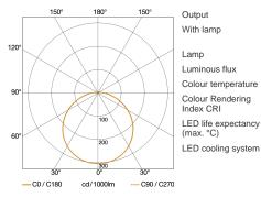
26 W Yes, STEINEL LED system LED cannot be replaced 1950 Im 3000 K 80-89 cy 70000 h m Active Thermo Control
