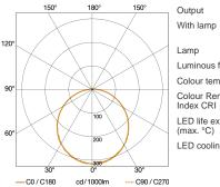
Luminous flux Colour temperature Colour Rendering Index CRI LED life expectancy (max. °C) LED cooling system 14 W Yes, STEINEL LED system LED cannot be replaced 1430 lm 3000 K 80-89
