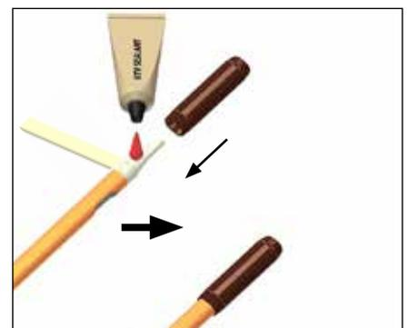
**4f.** Tape bus wires individually and then together. Continue taping to cover overjacket. Fill the end cap with RTV sealant and apply a circumferential bead to cable [minimum of 3 mm (0.12") wide]. Slide end cap onto end of cable.
