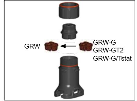
For HPT and FP cable exchange grommet supplied in Terminator kit with:
