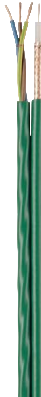
Prod.-Nr. 1871 Studioschaltkabel Studio connecting cable 0,6/3,7+ LiY 3 x 0,75 mm 2 – PVC parallel
