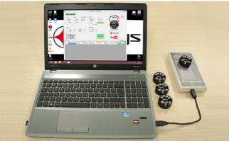
To configure this signal converter it is necessary to use a **RF Programmer** and the configuration software **LabSoftView**, available for all Pixsys parametric devices. After connecting the RF Programmer via USB and activating the software, it is possible in "EDIT" mode to configure the device selecting type of sensor, measuring range, output for error signal and sampling frequency for the registration. The keys "WRITE" and "READ" allow to write and read data on the devices quickly and easily.
