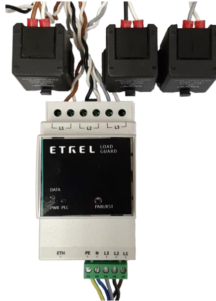
Figure 5: Load Guard with connected measuring current transformers
