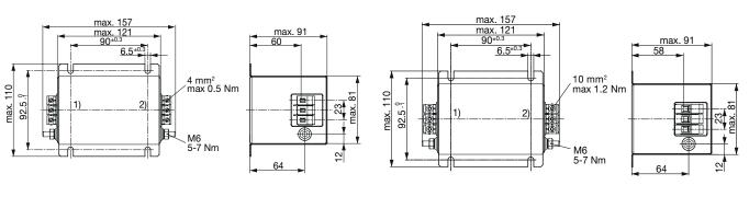
1) Line 2) Load Case 4B-10 1) Line 2) Load Case 4B-16
