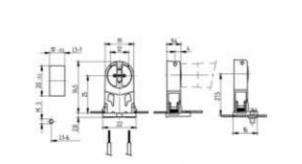
L1-1/L1-6: Recommended dimension - The distance between the cut-outs and the tolerance should be governed by the dimensions of the respective lamps and luminaires.
