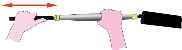
5. Put the shrinkable sleeve over the splice. Push the other conductor into splice until it stops. Pull conductors strongly out of splice.
