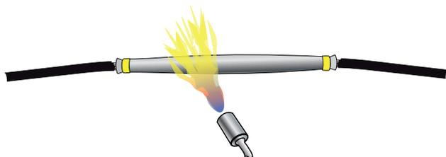
7. Warm the splice and conductors carefully.
