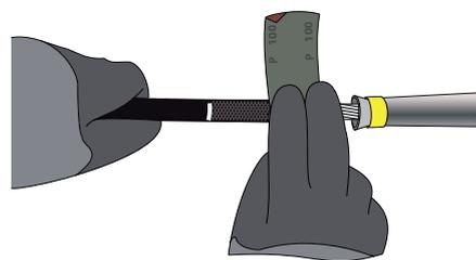
6. Roughen the insulation on the area which comes under the sleeve. Clean possible grease and dirt from the splice and the conductors.
