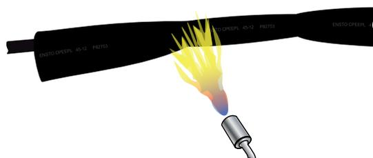
9. Center the sleeve over the splice and shrink it starting from the center. Continue shrinking to the ends of sleeve until the glue comes out.
