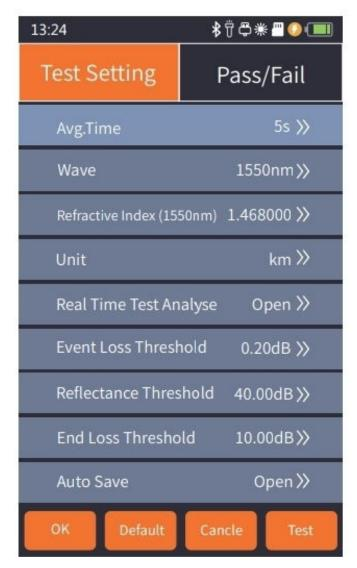
**Test Setting:** Avg.Time, Wave and Refractice Index are the same as those in Auto OTDR.
