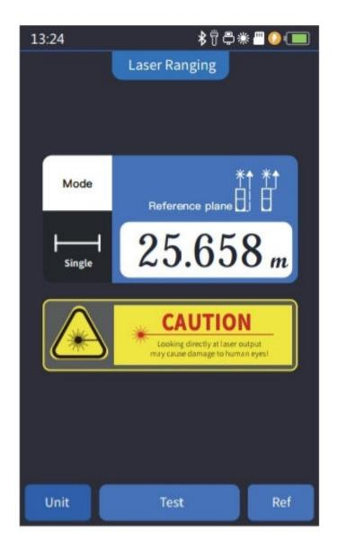
Laser Range: the maximum test distance is 40 meters Mode:Single/Continuous
