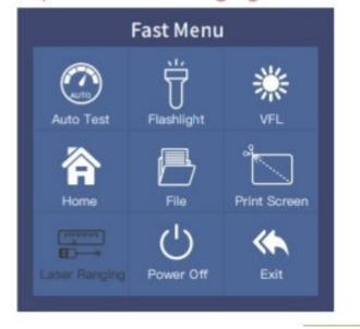
Press the " $\equiv$ " icon at the bottom of the screen to enter the quick operation menu, and press different function icons to enter the corresponding function interface or realize the corresponding operation functions.
