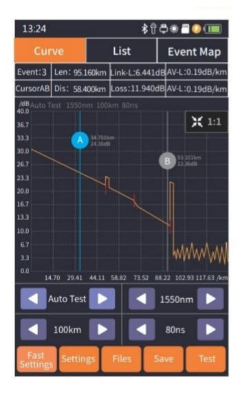
**Expert OTDR:** set parameters such as wavelength, range and pulse width.
