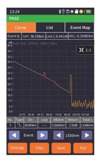
Auto OTDR: only need to set the wavelength, other parameters are automatically selected.
