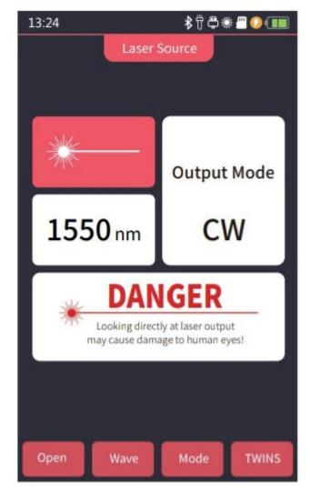
The wavelength of stabilized laser source is the same as OTDR wavelength. It is used to measure the parameters of telecommunication, CATV, LAN cable, insertion loss, isolation loss and echo loss of optical passive devices, and wavelength responsiveness of detectors.
