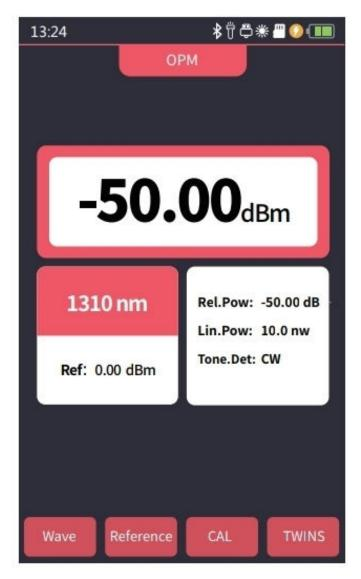
The function is used to test the power of optical signal and insertion loss of various devices and optoelectronic components. It can identify and measure the frequency of 270/330/1000/2000Hz optical signal.
