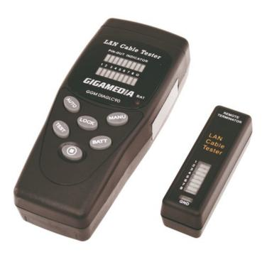
The remote cable tester is a versatile and rugged hand held tester designed for testing UTP, ScTP and SSTP cable for opens, shorts, reversals, miss-wiring and split pairs.
