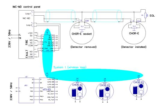
The IMC-MD system is wireless connected by UWI as one detector/node into uCU-IQ system (another CHOR-IQ alike) The Fire alarm or Fault of the uCU-IQ is indicated also in IMC-MD system as Fire/Fault in the Loop2
