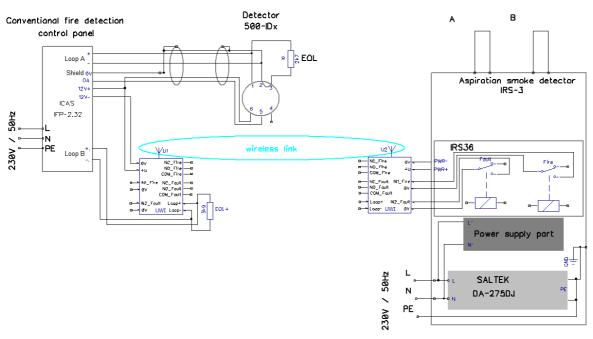
ICAS conventional pane IFP-2.32 and IRS-3 wireless conection by UWI with fire and fault indication in the loop B.
