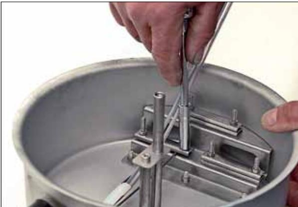
... and closing of strain relief clamp
