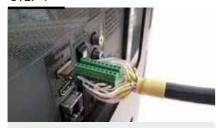
Connect the HDMI Male plug to a display (TV screen or video projector) and check that the cable works properly. In case of display problem, repair the connections as described in steps 4 and 5.
