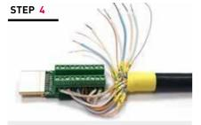
Link and screw the wires numbered from 10 to 19 on the corresponding screw terminals. Then, perform the same operation for connections from 1 to 9 and 20.
