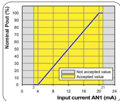
The reactive power limitation manages the output active power according to the current (4...20 mA) signal.
