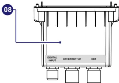
PVS-20/30/33-CCB must be connected to inverter USB connector (10) located under the Signals connection box (08).
