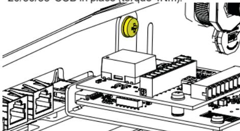
**⚠ ATTENTION** – The PVS-20/30/33-CCB, once installed, will be detected at the next restart of the inverter.
