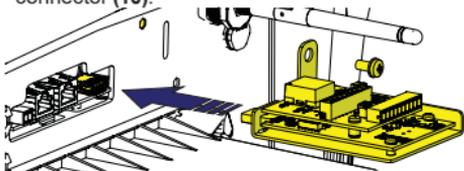
• Tighten the screw supplied to lock the PVS-20/30/33-CCB in place (torque 4Nm).
