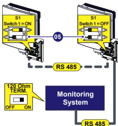
**NOTE** – The communication line must also be terminated on the first element of the chain which normally corresponds to the "third party system".
