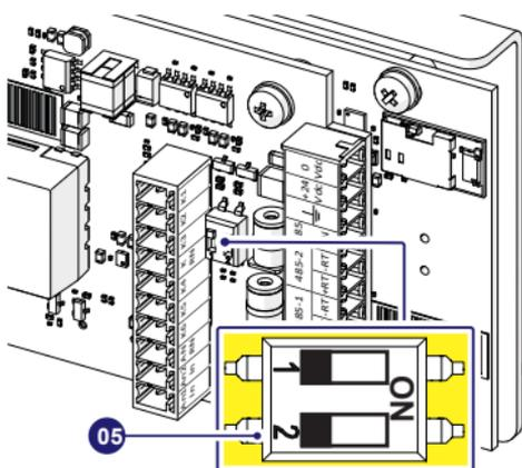
**NOTE** – Activate the termination resistance on the final unit of the chain.
