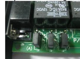
**Fig. 6 Jumper setting for ACTIVE CLOSE**
