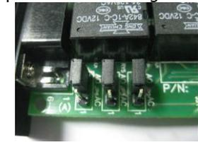
**Fig. 7 Jumper setting for ACTIVE OPEN**
