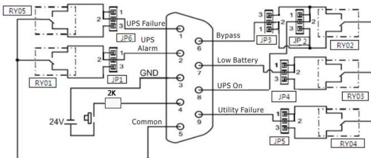
**Fig 2 Connection for ACTIVE CLOSE**
