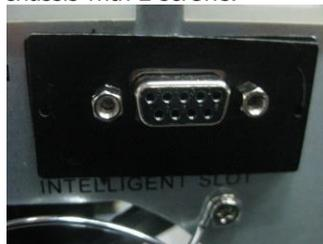
**Step 2:** Insert AS400 card into Intelligent Slot.
