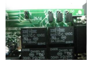
**Fig. 5 AO and AC silk printings indicates each 3-pin connector status**
