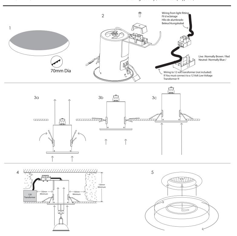
Astro Lighting downlighters are suitable for installation in gypsum wall board ceilings to timber floors that require up to 90min fire resistance to BS 476: Part 21: 1987 or BS EN 1365-2: 2000.
