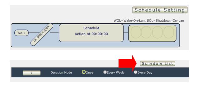
The schedule allows you to control the power outlet or turn ON / OFF/ RESET at assigned time
