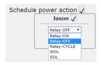
Once the scheduler has been Set Up , hit the "ADD No.:X Power Schedule" button and you will see your setting located on the bottom of the Action section .
