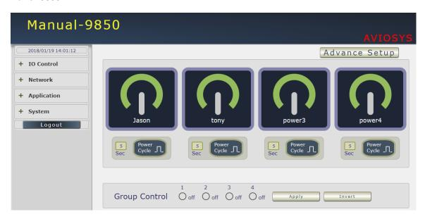
The IP Power 9850XX Console consists of six main sections which will be explained in details below.
