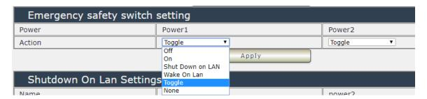
User can select different function of the individual button as OFF, ON, Shutdown on Lan , Wake On Lan , Toggle and None( Disable ) .
