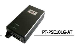
PT-PSE101G-AT is designed for indoor use. It works with input voltage of 100-240Vac. It has detection chip inside, which will detect and classify PD before powering it. It will not apply power until a standard-compliant PD is detected. The effective distance is 100 meters over Cat5e/Cat6 cables.
