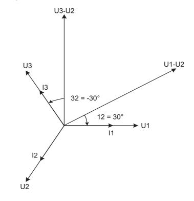
a pure resistive load where the phase currents are in phase with its respective phase voltages.
