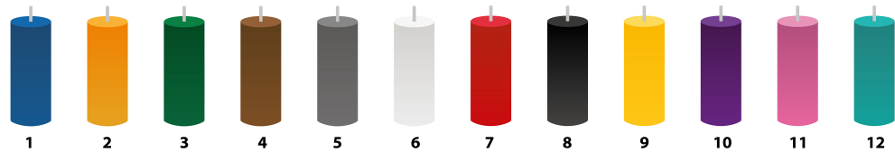
Colour coding (as per TIA-598-C)
