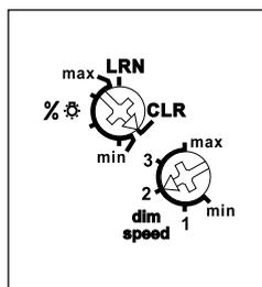
The flashing of the LED as soon as a new setting range has been reached when turning the rotary switch helps to find the desired position reliably.
