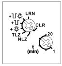
With the top rotary switch in the setting LRN up to 35 wireless pushbuttons and/or wireless motion/brightness sensors FBH can be assigned of which one ore more central pushbuttons. The required function of this staircase off-delay timer can then be selected.
