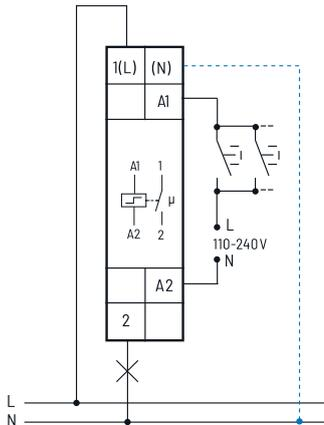
If N is connected, the zero passage switching is active.
